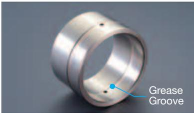
The HN bushing containing High-viscosity oil is provided at each joint to reduce grease consumption, extend lubrication intervals (100 to 500 hours), and increase durability.
