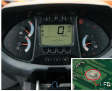
On the indicators, monitors and alarms, many LEDs are utilized for longer service life resulting in less failure, enhancing the reliability.
