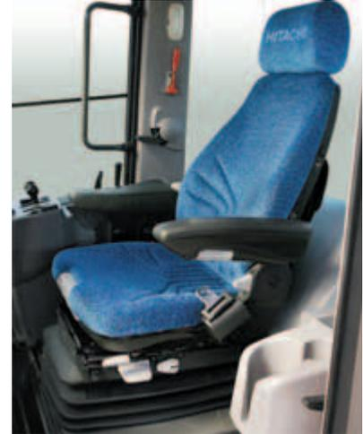
The air suspension seat can be adjusted in multiple ways: weight-height, fore-aft position, backrest tilt, and armrest angle, seat cushion length and angle, headrest height and angle adjustment, lumbar support. Seat heater is equipped as standard.
