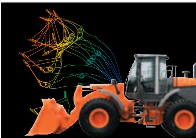
With the new parallel/tandem circuits, the lift arm and bucket can be operated at the same time, unlike conventional machines. This can remarkably increase digging and loading efficiency for higher production.
