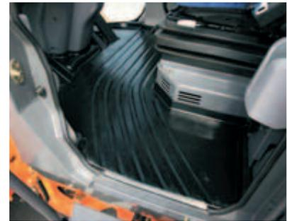
The cab floor is stepless (flat) for ease of cleaning.
