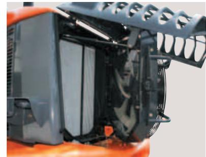
The rotation of the hydraulically operated cooling fan with heat-sensing system can be reversed for easy removal of dirt from the radiator. The fan itself can swing open for easy cleaning.
