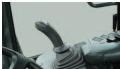
The multi-functional joystick lever is provided atop of the control lever for operating ease.
