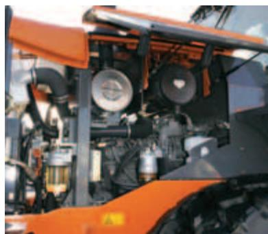
Dual fuel filters with sedimentary function and engine oil filter are strategically located for the convenient daily inspection and servicing from the ground.
