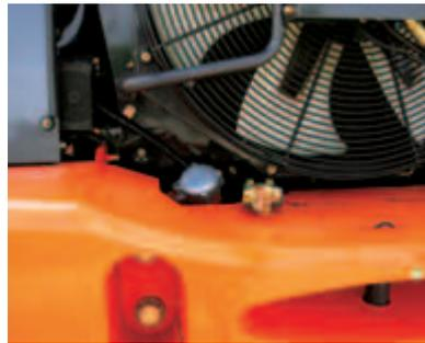
The fuel supply port is located for convenient fuel supply from the ground.
