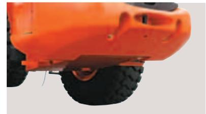
The large counterweight is arranged to protect the fuel tank from collisions with obstacles during operation.
