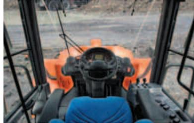
The panoramic cab gives almost all-round visibility with the widened front glass window and pillar less cab rear corners. Front wheels are always in the operator's vision, enhancing safety and increasing loading efficiency.
