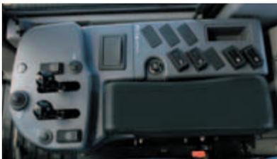
Switches and controls are efficiently laid out in the right console for ease of operation.
