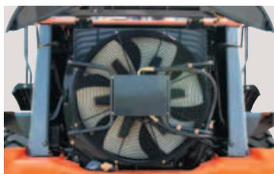
The cooling fan is enclosed by a full guard (metal net) to protect service technicians from injury during servicing and maintenance.
