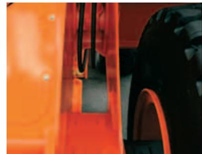
The DL front frame is shaped for easy removal of dirt, stones and snow.
