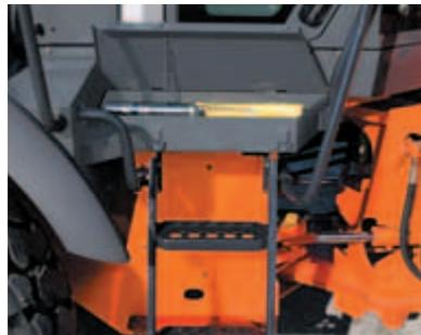
A large tool box is provided at the top step of the ladder on the right side of the machine. The tool box can hold a grease gun and tool kit.
