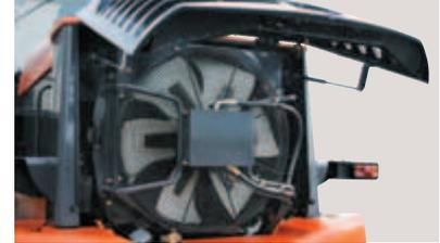
Fan speed can be adjusted depending on fluid temperature to effectively cool down coolant, hydraulic oil, transmission oil and torque converter oil. The result is extended component service life and reduction in fuel consumption. The fan is also separate from the engine for easy servicing.
